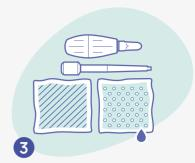
Remove the capillary and lancet from the Accessory Pack and remove the sterile gauze and alcohol wipe from their packaging.
